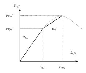
Figure 4. Bi-linier curve model for compression stressstrain paralel to the grain.
