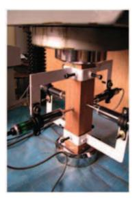
Figure 1. Compression parallel to the grain specimen under loading test.
