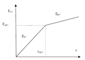
Figure 7. Bi-linier curve model for compression stressstrain perpendicular to the grain.
