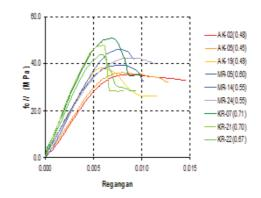
Figure 3. Typical compression stress-strain curve paralel to the grain.
