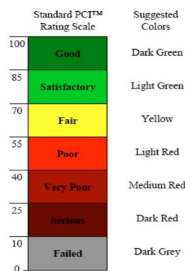
Gambar 7 Rating Kondisi Perkerasan Berdasarkan PCI (ASTM, 2007)
