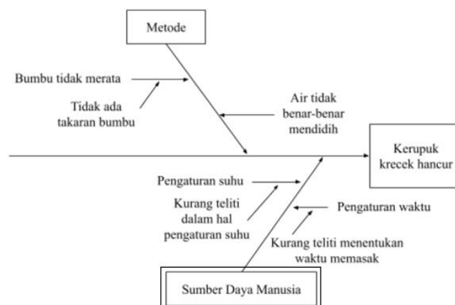
Figure 3. Cause-and-Effect-Diagram (Fishbone Diagram) Factors Causing Cracked Crackers (B)
