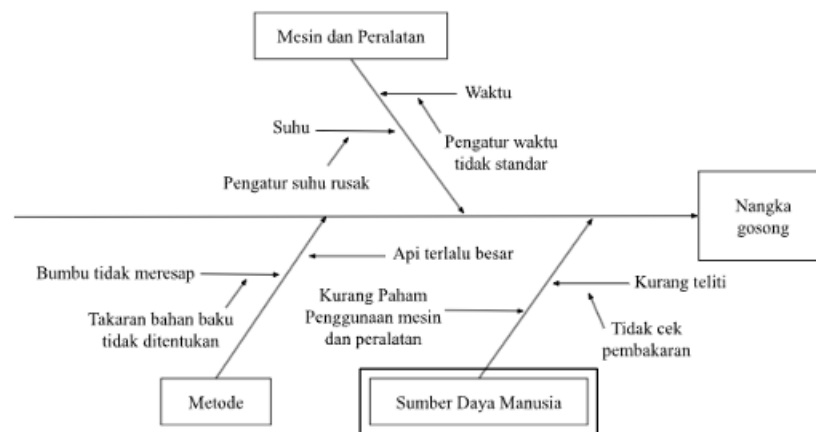
Figure 4. Cause-and-Effect-Diagram (Fishbone Diagram) Factors Causing Burnt Jackfruit (C)
