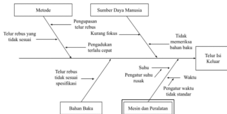
Figure 2. Cause-and-Effect-Diagram (Fishbone Diagram) Factors Causing Egg Fill Out (A)
