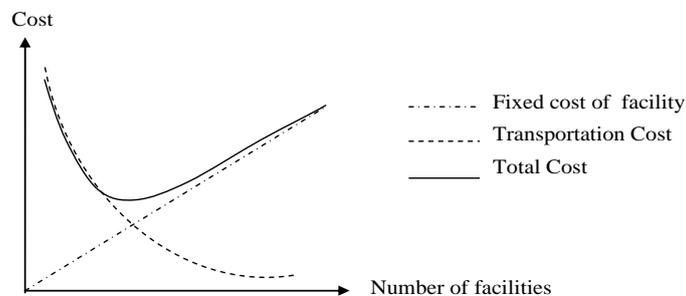
**Figure 6** Relation Between Transportation, Facility, and Total Cost
