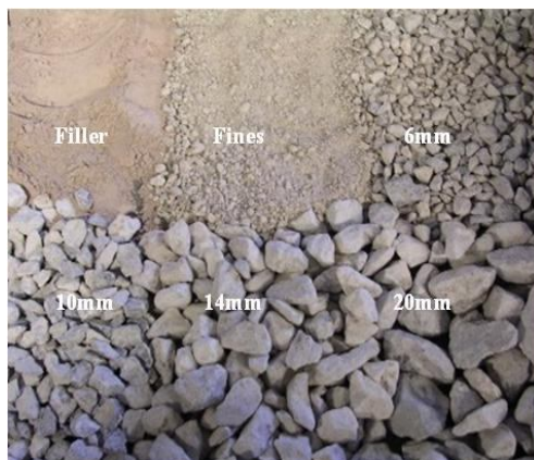
Figure 2a Virgin crushed limestone aggregate
