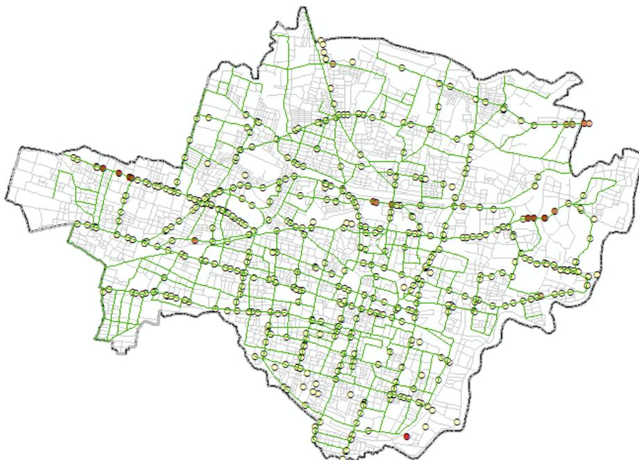
**Figure 5** Traffic Accident Blackspot (Using Hot Spot Analysis Method)
