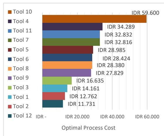
**Figure 4.** Optimal roughing process cost for each tool after removing deflection constraint
