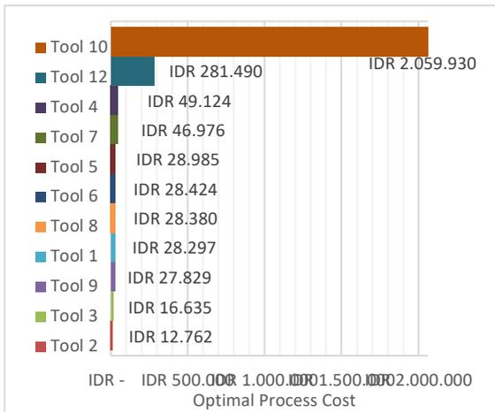
**Figure 2.** Optimal roughing process cost for each tool\*
