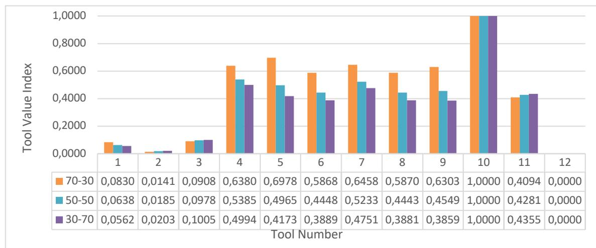
**Figure 5.** Cutting tool valuation result without deflection risk limit
