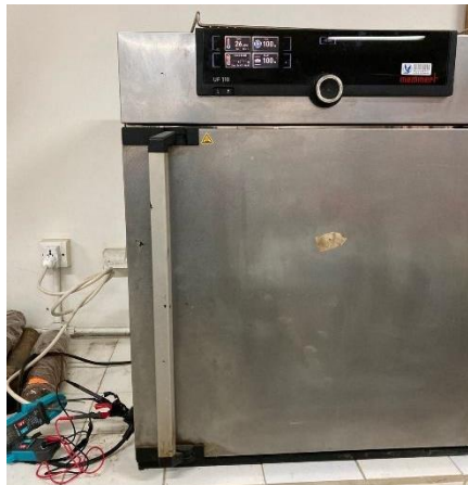
Figure 1. Electrical charge voltage and current measurement at the oven
