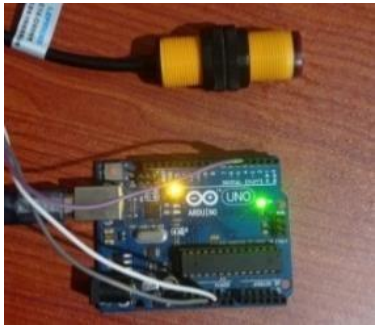
Gambar 8 Pengujian sensor Infrared Proximity E18-80NK
