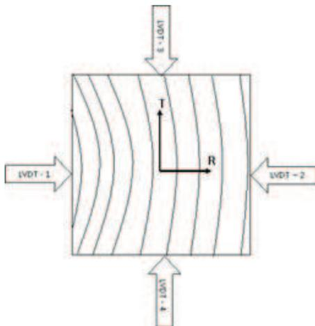
Figure 5. LVDT setting for radial and tangential direction.
