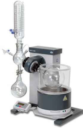
**Gambar 3.2** Evaporator vakum
