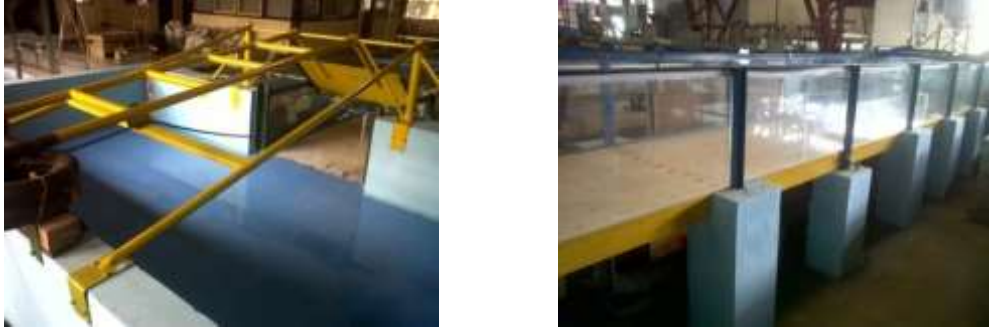
Figure 2: Reservoir and Gate (Left); Channel (Right) (Setiawati, 2011)
