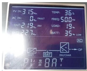
Gambar 6. Display monitor Off-Grid Solar Panel inverter
